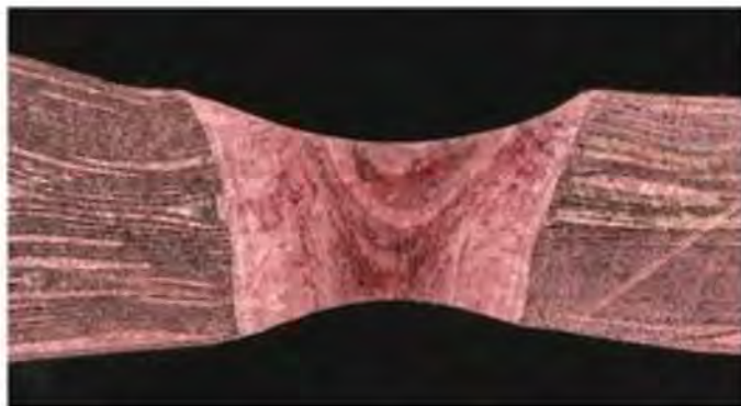
FIGURE 4. Shown in cross-section, 40 10- \mu\text{m} -thick copper foils are welded together using blue laser light.
